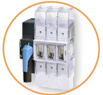
Terminal covers provide protection against accidental contact and phase separation of the switch, and Perforated holes allow for contact temperature monitoring without removing the covers
